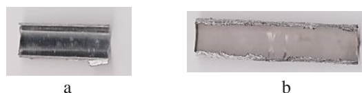
Figure 1. The photograph images of zirconium-niobium cladding tube a) no delay, b) with delay in rinsing step
