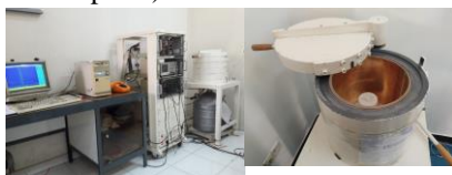
Figure 2. Gamma-ray spectroscopy systems in NAA laboratory
