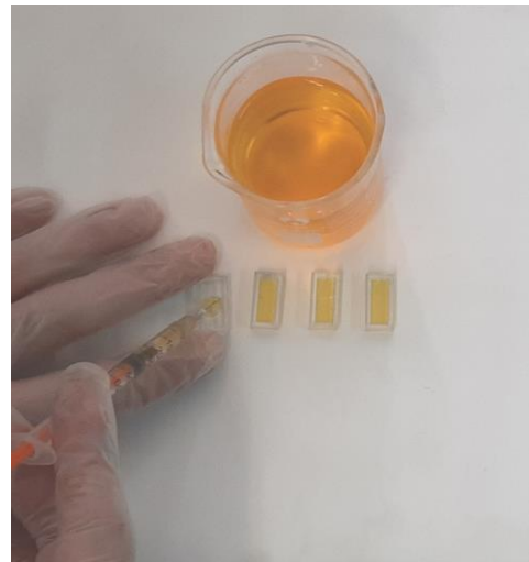
Figure 1. Filling step of Fricke agarose gel Layer dosimeters.
