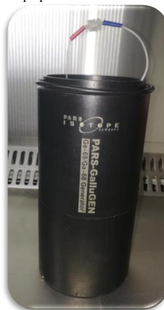
Figure 1. 70 mCi ^{68}\text{Ge}/^{68}\text{Ga} generator
