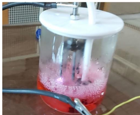
Figure 2. Pin-to-water corona discharge reactor.
