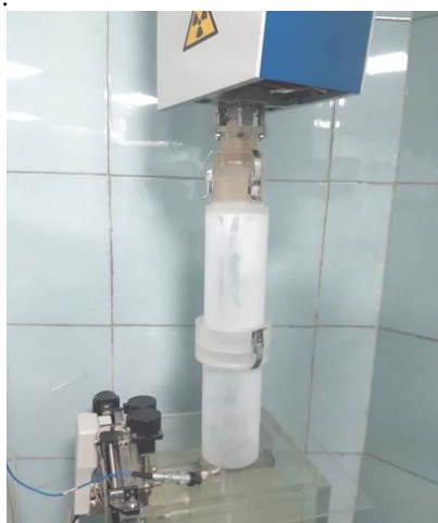
Figure 1. Experimental setup to measure dosimetry response of polymer/CNT nanocomposite using the LIAC dedicated IOERT machine.
