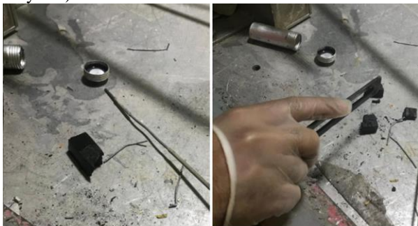
Figure 5. NBR damage after 1 day irradiation in neutron flux of 10^{13} n/s.cm 2
